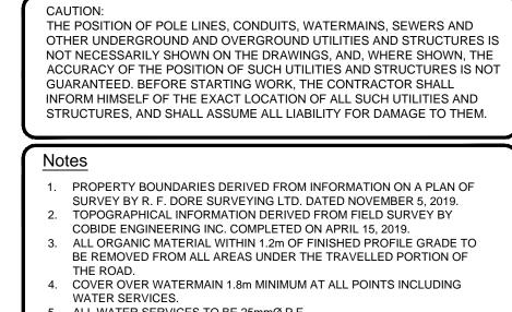
. ALL WATER SERVICES TO BE 25mmØ P.E. SANITARY SEWER TO BE PVC SDR 35 ALL STORM CATCHBASINS TO HAVE A MINIMUM SUMP OF 600mm
