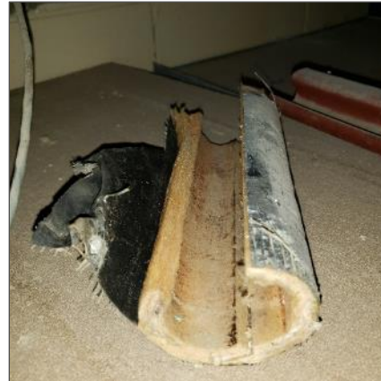
Non-asbestos black tar paper present underneath foil wrap on fiberglass pipe insulation, location 1.
