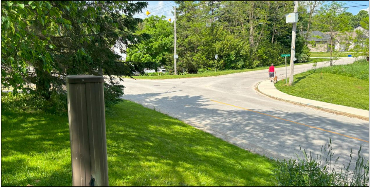
Figure 11: View of a motorist looking left from new driveway (10 m back) – Approach sight distance (TNS, 2024).
