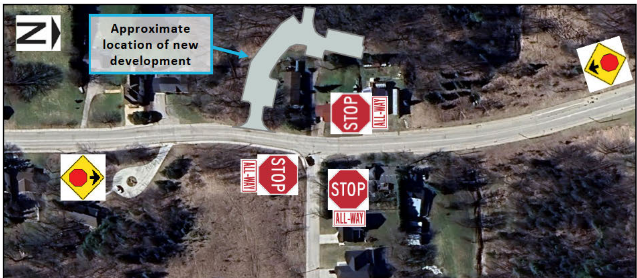
Figure 14: Signage for an AWS conversion at Yonge Street North and Valleyside Drive.
